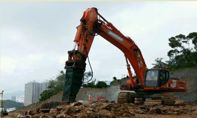
Heads of breakers are wrapped by acoustic materials to lower the noise level.
