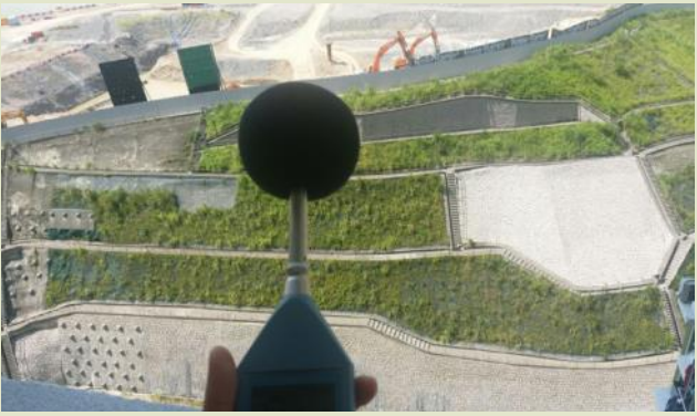
Noise measuring are implemented regularly in nearby housing estates such as On Tat Estate, On Tai Estate and Po Tat Estate. Construction noise generated by the works are being monitored in a proactive way.
